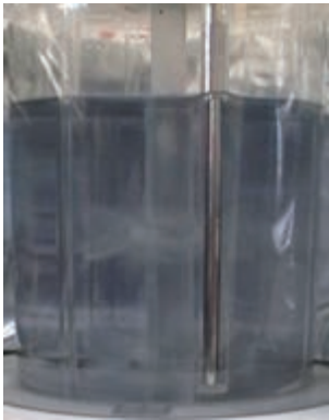
Figure 7: Determining the mixing time based on the decolourisation method using a video camera. Specified is the time after addition of sodium thiosulfate, 0 seconds is the moment of addition.
