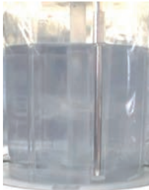
Figure 7: Determining the mixing time based on the decolourisation method using a video camera. Specified is the time after addition of sodium thiosulfate, 0 seconds is the moment of addition.
